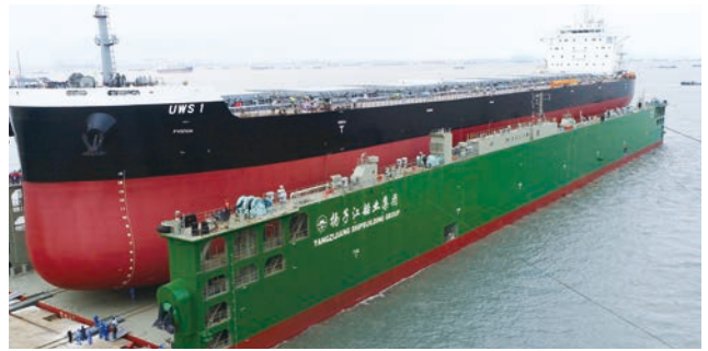
▲ 浮船坞 (最大滚装举力 23,500T) Floating Dock (Max roll-on lifting capacity: 23,500T)
